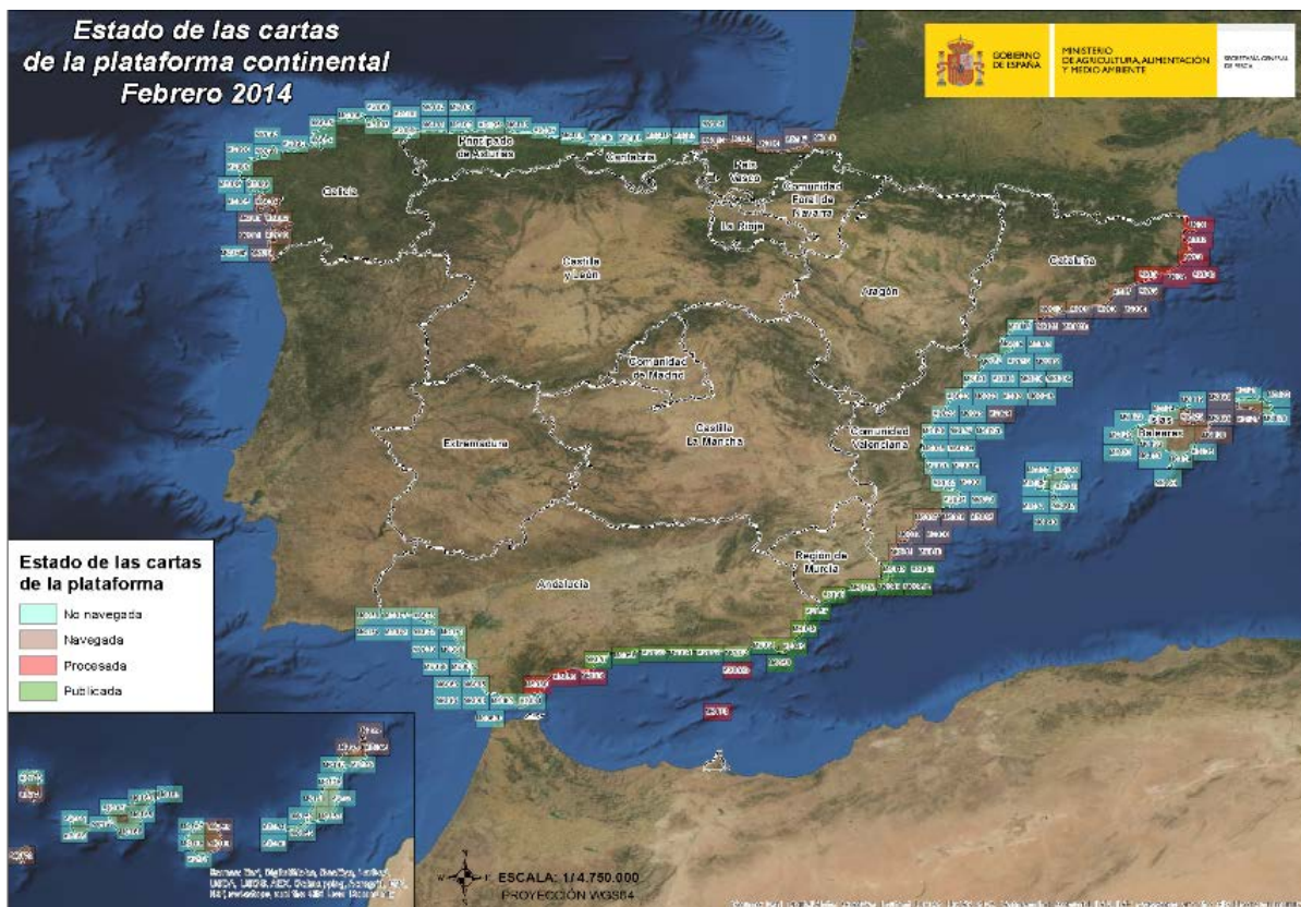
Figure 19. Distribution of map sheets in the Iberian Peninsula and Canary Archipelago. Green rectangles, indicate published maps; red colour indicate that the datasets have being processes; pink rectangles refer to surveyed areas; and blue rectangles indicate areas not surveyed.
