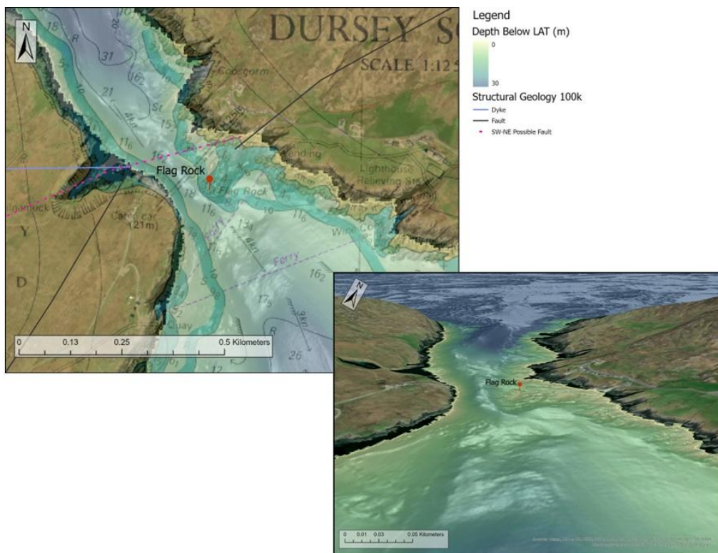
Figure 7: Nautical chart with bathymetry underlain and Flag Rock indicated (left), and 3D image looking north-west through the sound and Flag Rock indicated (right).
