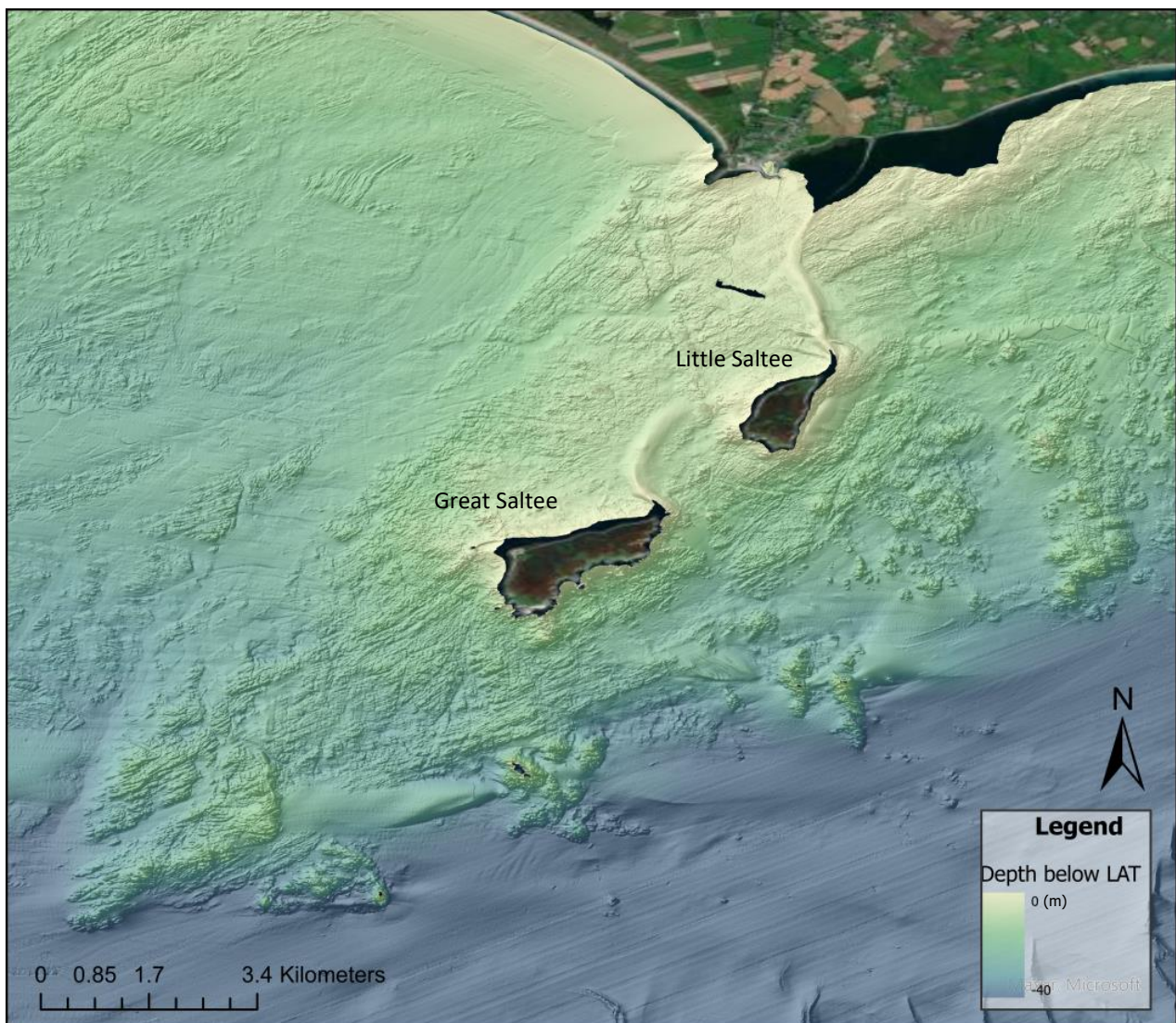
Figure 1: Bathymetry of the Saltee Islands. Depths are given as negative below Lowest Astronomical Tide (LAT), and positive above LAT.
